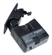
The Schneider Electric range of current transducers delivers high performance, reliable current monitoring for applications including fan status, belt loss, and most Variable Speed Drive (VSD) applications. Current transducers detect changes in a conductor's current/amperage and provide an analog output to Building Management System (BMS) controllers. The current transducers are available in solid-core versions for new projects and split-core versions to accommodate retrofits.
